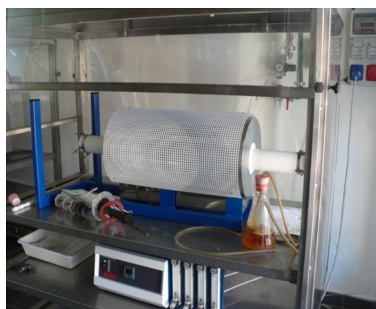
Tubular Lenton furnace, used for the batch thermal treatments
